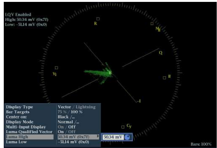
Figure 20. Tektronix's Luma Qualified Vectorscopes are an exclusive feature that allow you to show a vectorscope image for a specific tonal range. In this case, only up to 50 mv. So this is showing the shadows or darkest parts of the image.
