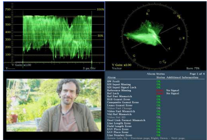
Figure 4. The Waveform Monitor shows that the image doesn't take advantage of the full dynamic range. Blacks are lifted (above 0) and whites aren't at 100% (or 700 mv).
